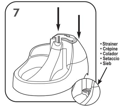
**7. Replace filter reservoir unit. Reservoir locks strainer into place.**
