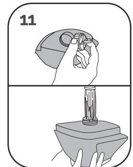
**11. Remove cap from water reservoir, fill with water and replace cap.**
