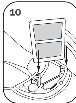
**10. Insert filter in corner slots of filter reservoir. Slide it down to bottom.**
