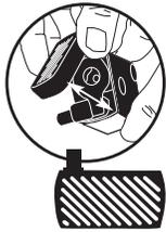
**Before Proceeding:** be sure pump intake cover is snapped on securely.
