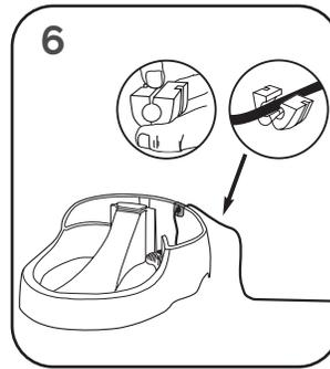
**6. Open grommet and close around power cord. Insert grommet into base.**
